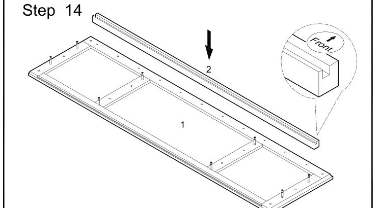
Attach slat (2) to top panel (1) using dowels as guides. Note the direction of slat (2) as shown above.
